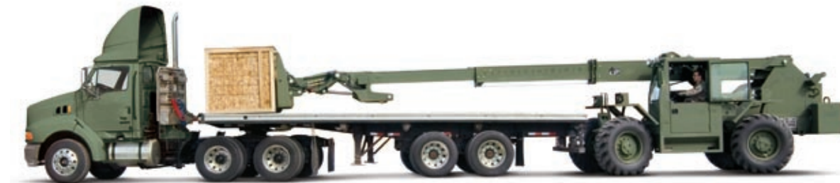
With its extended reach and deep access, the ATLAS II can load or unload palletized material from containers located either on the ground or on trucks.
